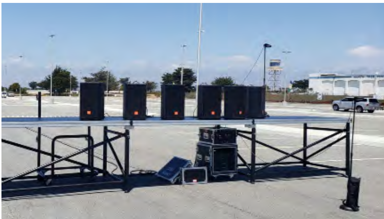
The delay tower 265 feet in front of the main PA System.
